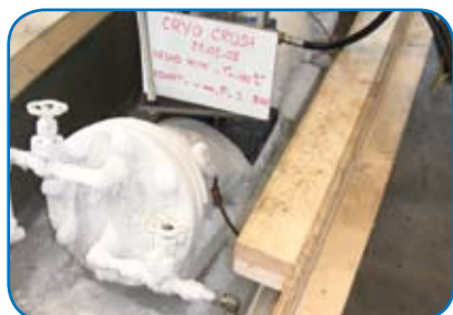
8" Multi-LNG White STS crushed with external loads up to 160 kN. Internal hose pressure of 6 bar. Done both ambient and cryo- genic without any leakage.
