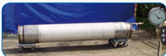
Ambient burst test on prototype Multi-LNG White 16"
